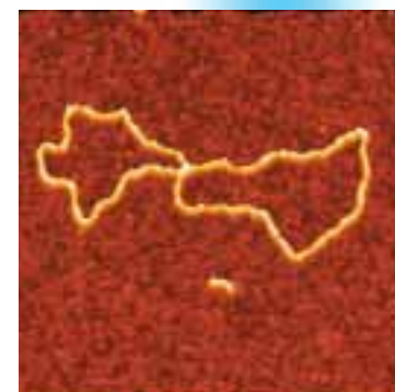
DNA plasmid on a mica substrate AC mode measurement in air
